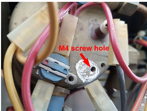
Figure 3. Two examples of boilers with M4 screw holes at where thermostats are installed.
